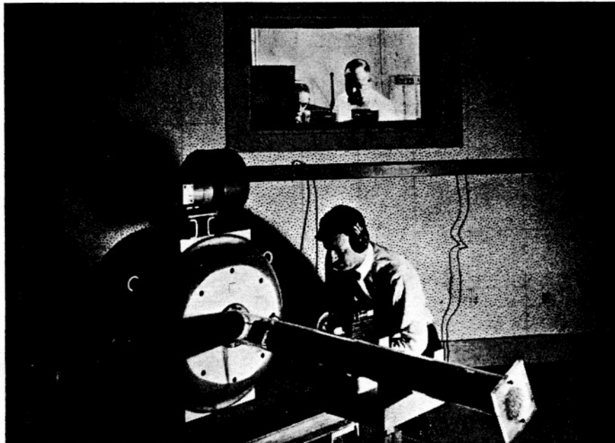
Avco acoustic noise generator subjects a nose cone component to as much as 170 db in progressive wave tube.
